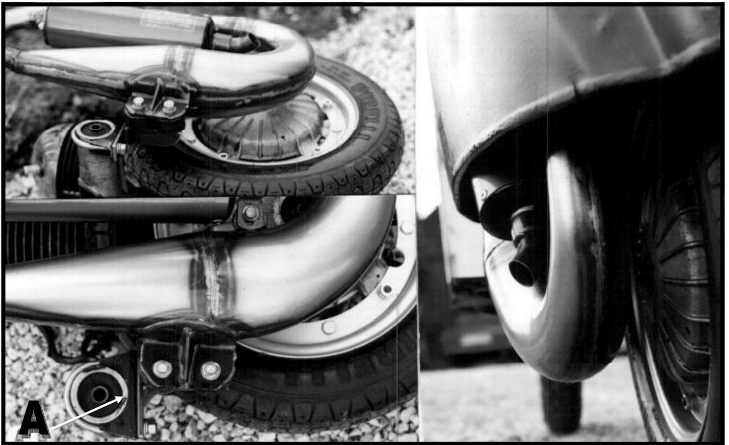
When fitted correctly, the clamp edge should be level with the end of the engine arm.
